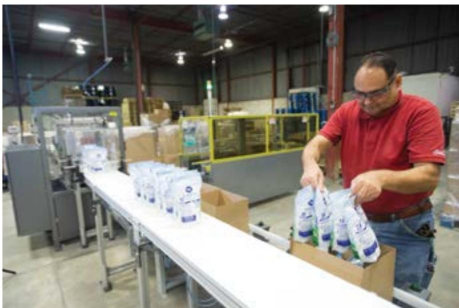
Filled stand-up pouches travel alongside corrugated shipping cases coming out of the Eagle Packaging case-erector to the line operator to be inserted inside the boxes.
