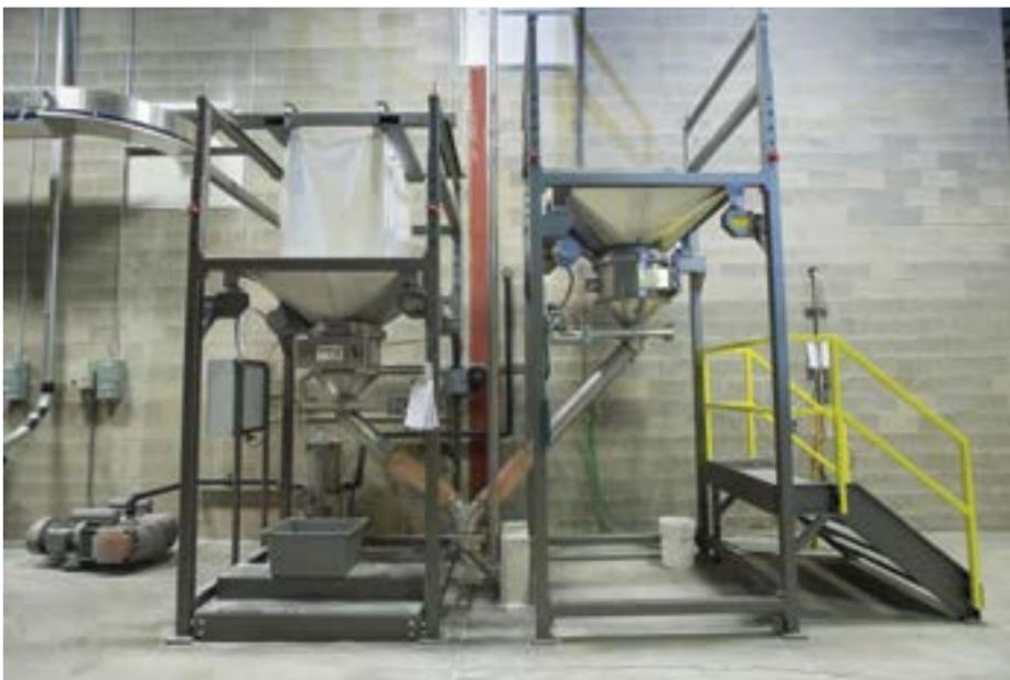
A heavy-duty bulk discharger and bucket elevators from UniTrak Corporation are used to transfer bulk powder up to the automatic weigh scales on the mezzanine level above.
