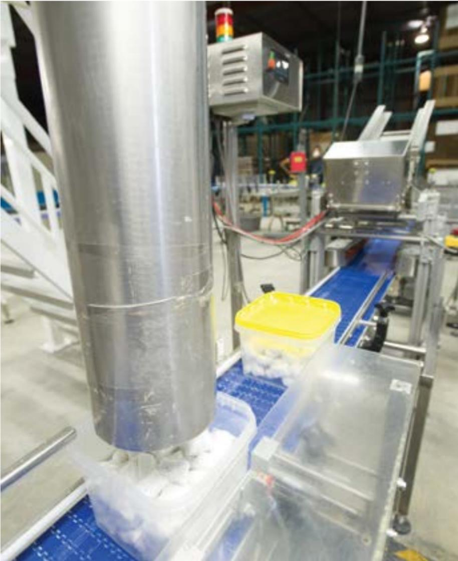
A transfer tube connected to Multiweigh scales overhead dispenses precise quantities of dishwash detergent pods into plastic tubs transferred by the Speedway conveyors below.
