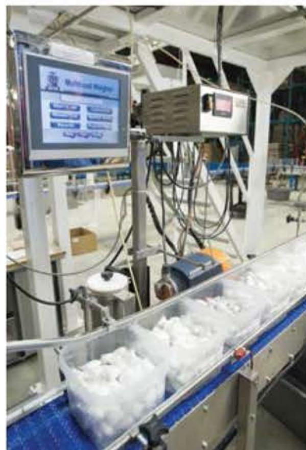
Each filled plastic tub traveling on top of the Speedway plastic conveyors is checked for weight and quantity by the Multiweigh checkweighers prior to lidding and labeling.
